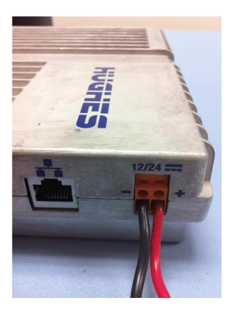
Figure 4-9 - Connecting power leads
