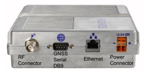
Figure 1-7 – Back side view of IDU
